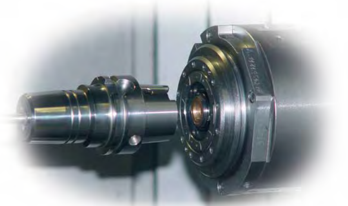
Fig. 1: HSK-A 63 interface, automatic tool change
