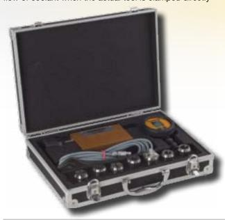
in the stationary tool spindle. This way, it is possible to establish the real conditions of the relevant machine and tool configuration and measure the resulting actual rate of flow.
