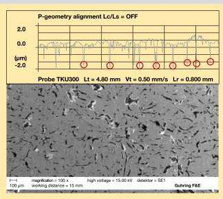
Homogenous cast structure with even distribution of casting cavities. HR 500 CAST continues to achieve a surface quality of Ra 0.46 after a tool life of approximately 60 m.
