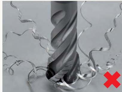
Thread chips can cause tool breakage
