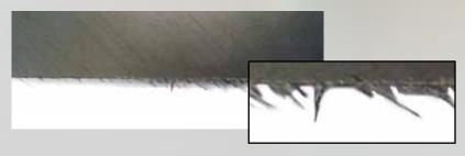
Milled CFRP workpiece edge without delamination machined with a Guhring CR 100 end mill
