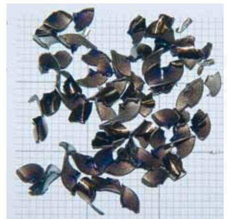
Fig. 3: Problem-free chips preventing chip congestion and jamming of the tool.
