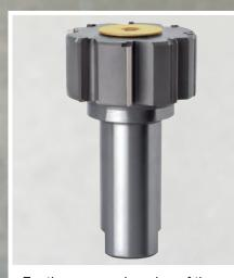
For the secure clamping of the HR 500 GT tool head the straight shank is also fitted with a tang. Of course, a precise clamping is also possible in hydraulic chucks with standard length.
